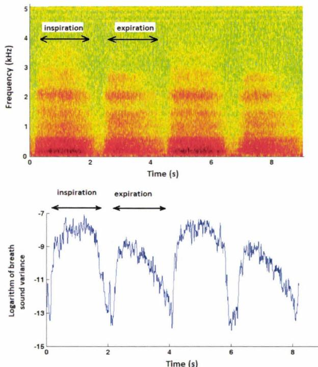
Figure 1. The spectrogram of an example breath sound (top) and the logarithm of sound variance used to separate the phases (bottom).
